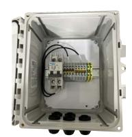
11.41' H x 10.68" W x 6.36" D NEMA 4X junction box with DIN rail mounted circuit protection and terminal strip, pre-mounted cable glands
