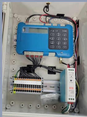
IC4C panel with power supply, terminal strip, plug and play load cell connection
